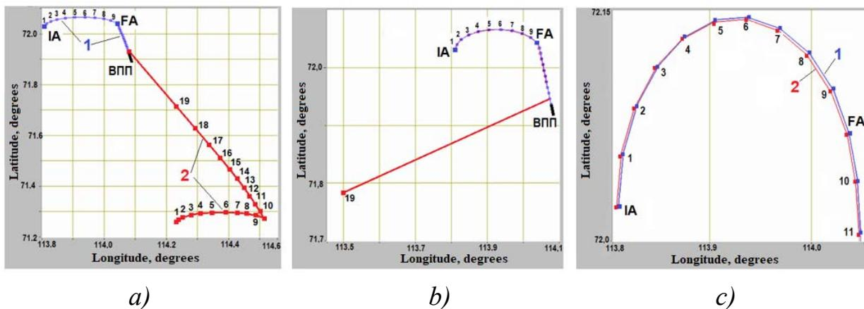
Fig.3 UAV and aircraft flight trajectory in horizontal plane
